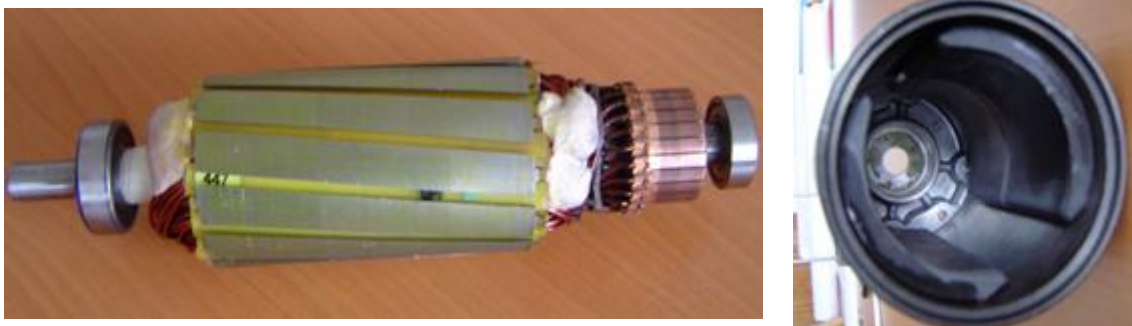
Fig. 1: Rotor and stator of original motor.
